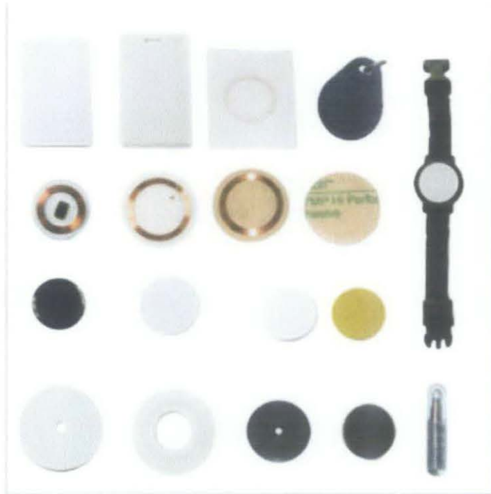
Figure 7: Passive RFID Tags in Various Form Factors [9]
