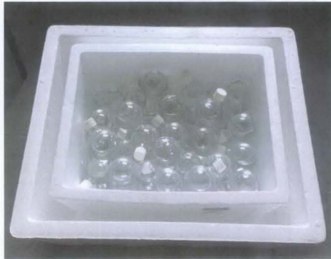
Figure 17: TES filled with encapsulated ice storage
