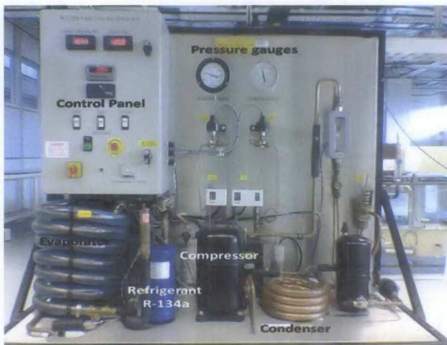
Figure 10: Laboratory water chiller
