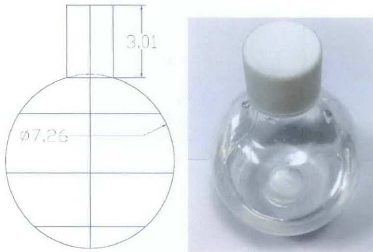
Figure 16: Encapsulated storage container in (cm)
