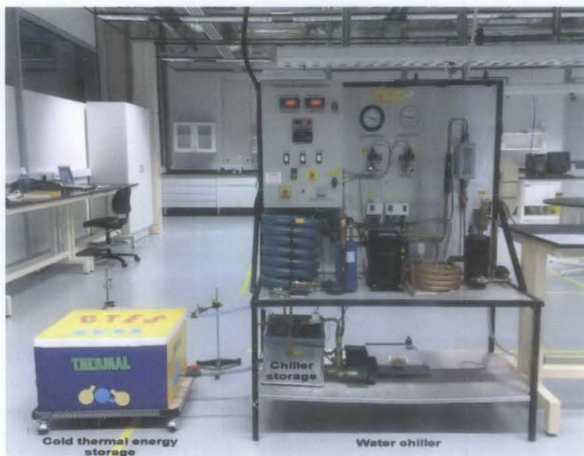
Figure 22: CTES and water chiller
