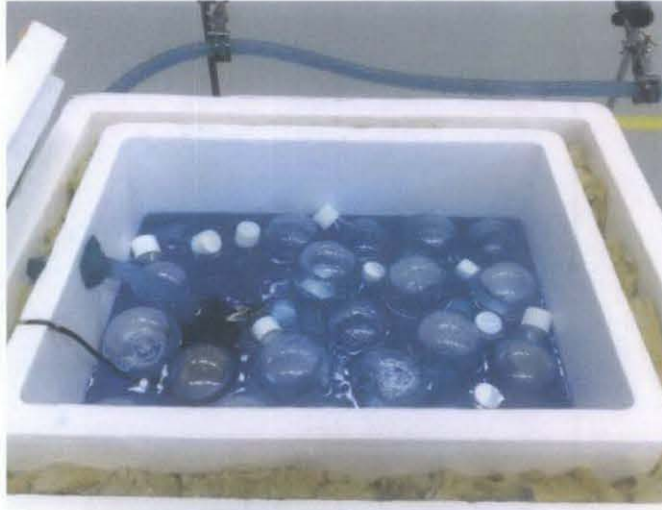
Figure 20: Rock wool insulation at gaps
