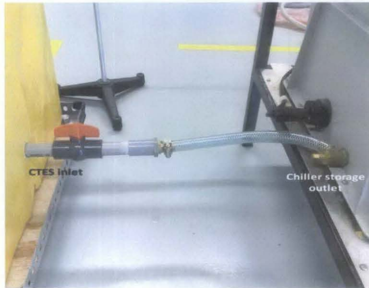
Figure 14: Connection from chiller storage to CTES
