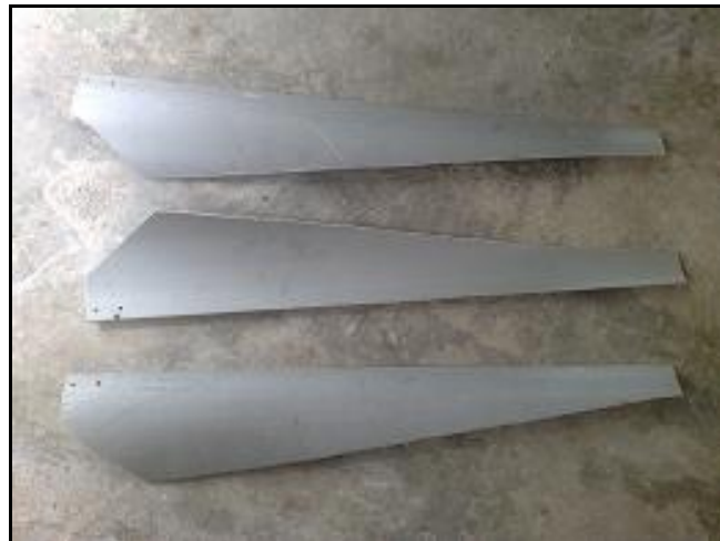
Figure 17 : Blades made from 6" PVC
