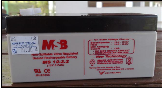
Figure 3 : 12V 3.2AH lead acid batteries
