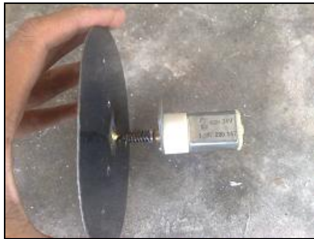
Figure 19 : Welded metal hub and geared motor
