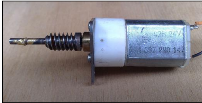
Figure 10 : 24V DC Generator
