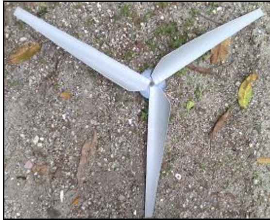
Figure 20 : Assembled PVC blades and metal hub
