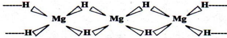
Figure 4.1 Schematic representation of solid phase \text{MgH}_2
