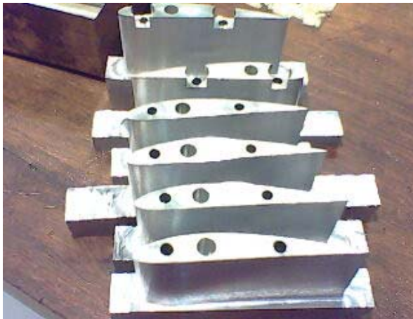
Figure 5.8: NACA 4412 Model in Sections
