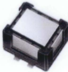
Figure 7 : A MURATA IRS-A200ST01-R1 PIR sensor
