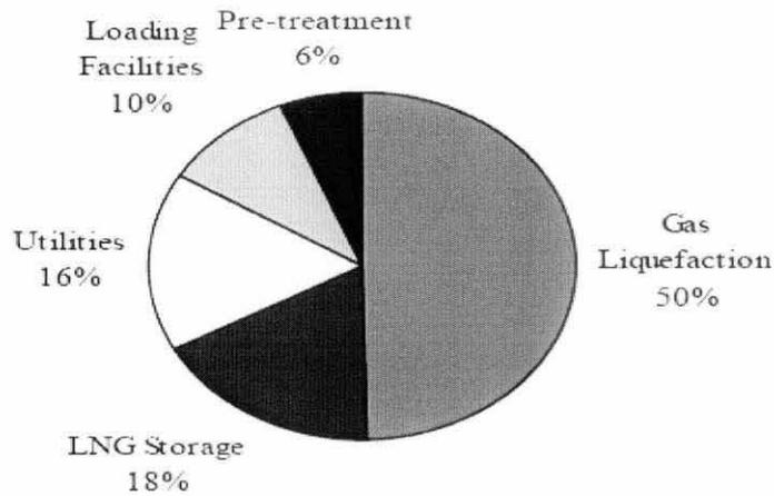
**Figure 2: Typical breakdown of liquefaction plant capital costs [2]**
