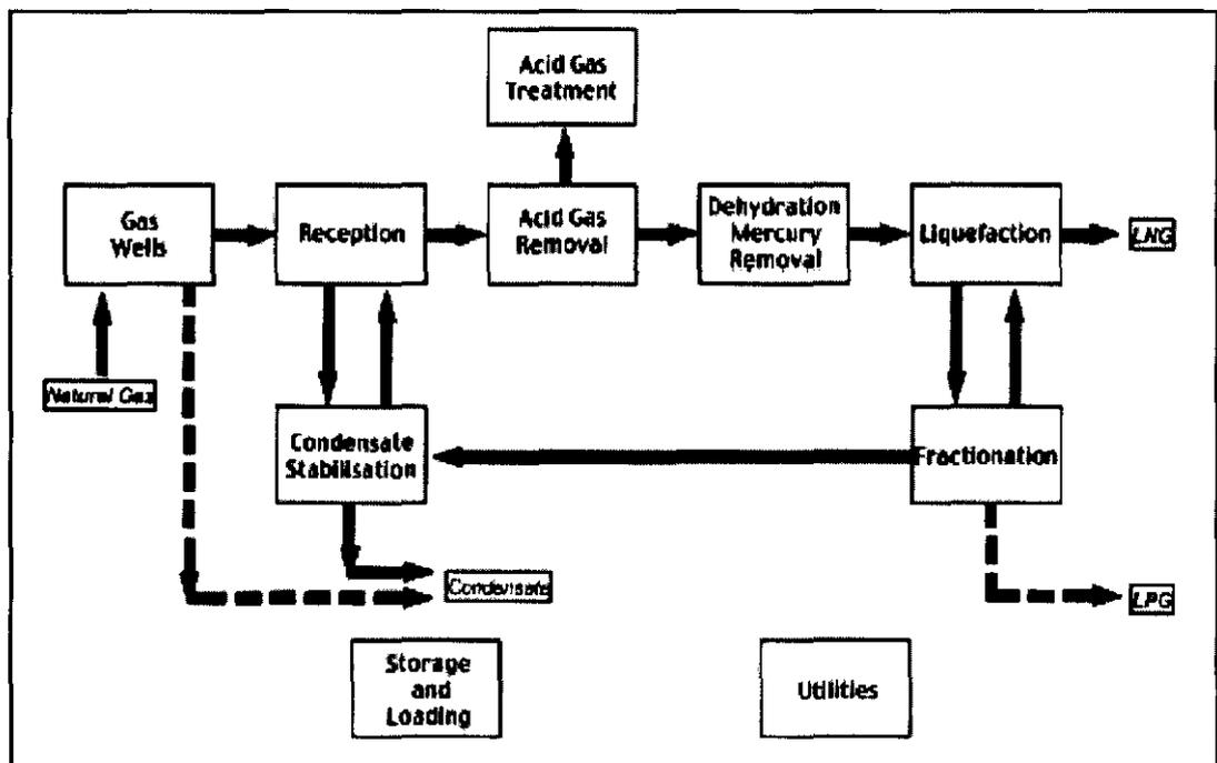
Figure 5: LNG block flow diagram [5]
