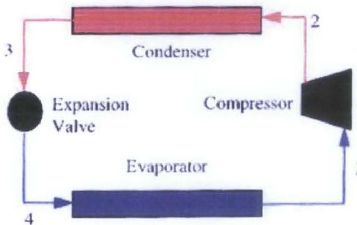
Figure 6: Refrigeration cycle [6]
