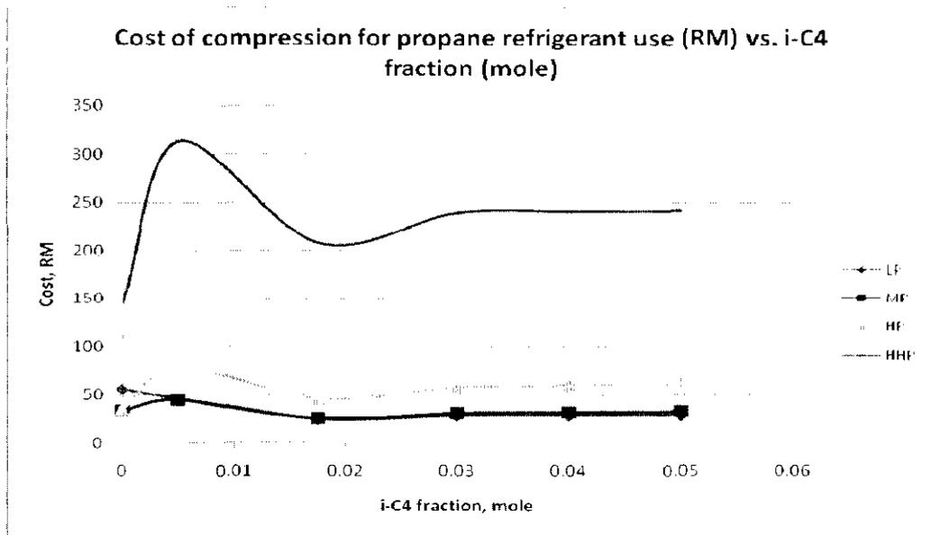
**Figure 52: Graph of cost of compression for propane refrigerant use vs. i-C4 fraction**
