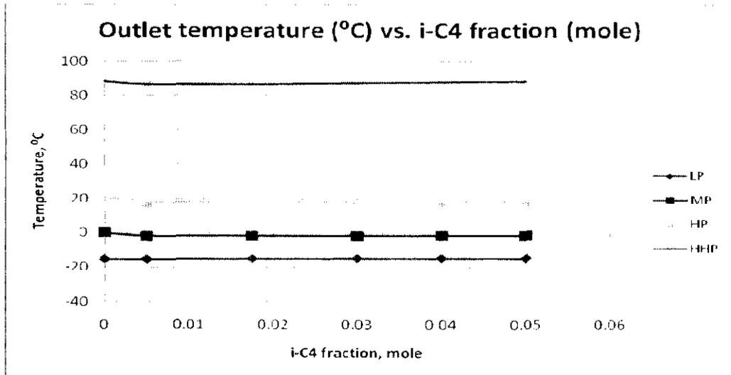
**Figure 30: Graph of outlet temperature vs. i-C4 fraction**
