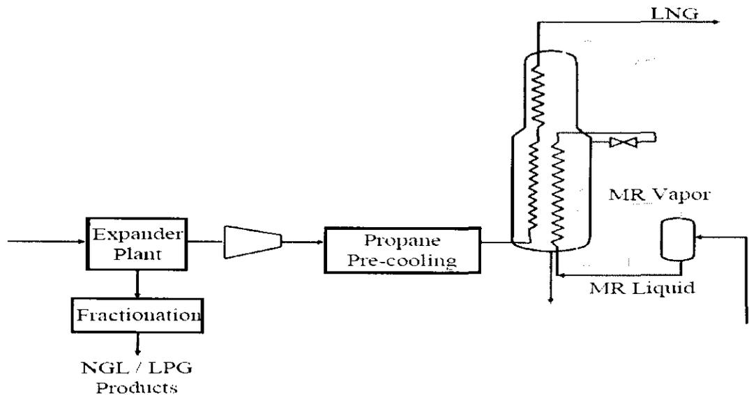
**Figure 10: NGL/LPG extraction before liquefaction unit**
