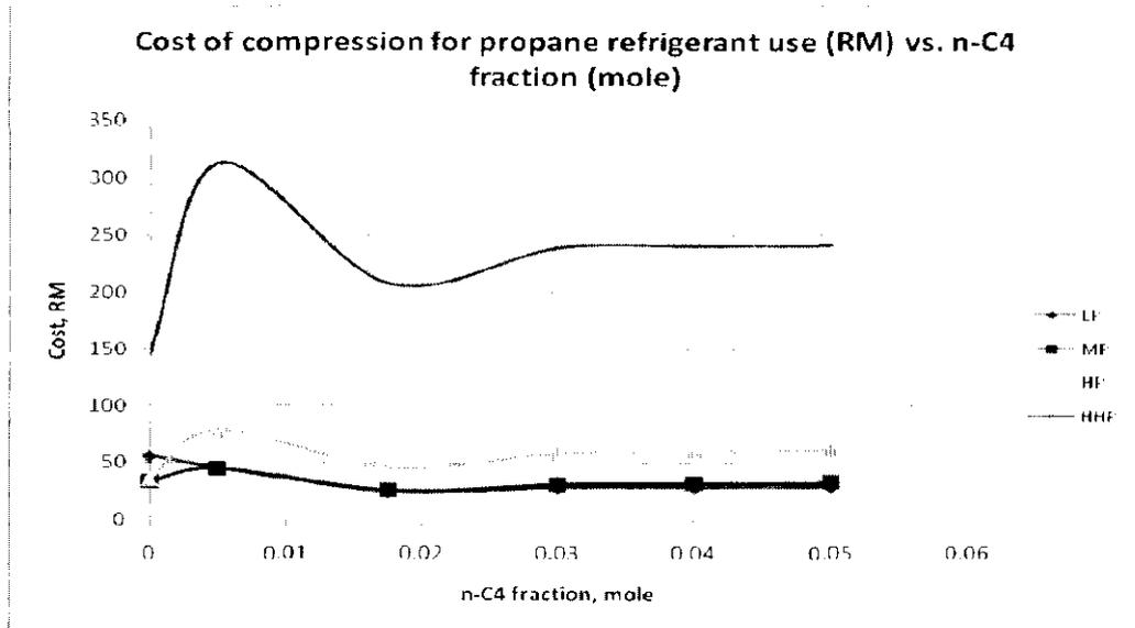
**Figure 51: Graph of cost of compression for propane refrigerant use vs. n-C4 fraction**
