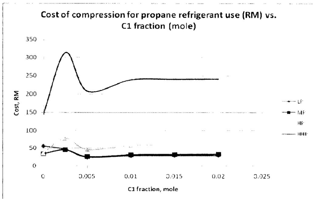
Figure 48: Graph of cost of compression for propane refrigerant use vs. C1 fraction
