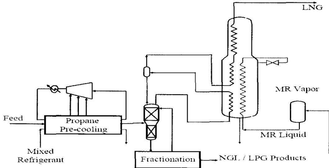
**Figure 11: NGL/LPG extraction integrated with liquefaction unit**
