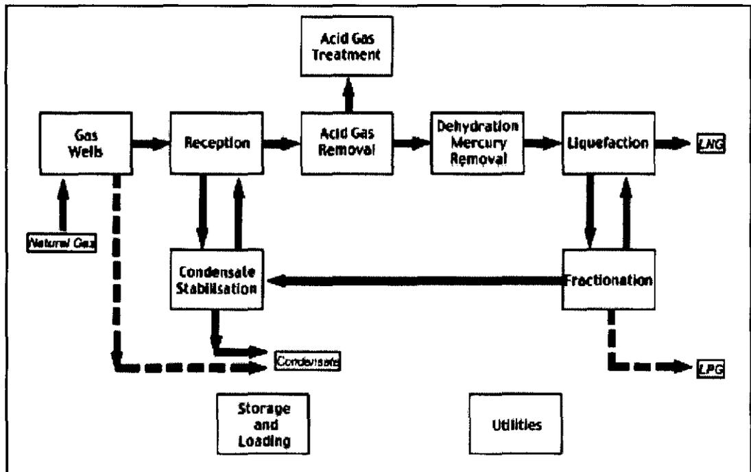
Figure 5: LNG block flow diagram [5]
