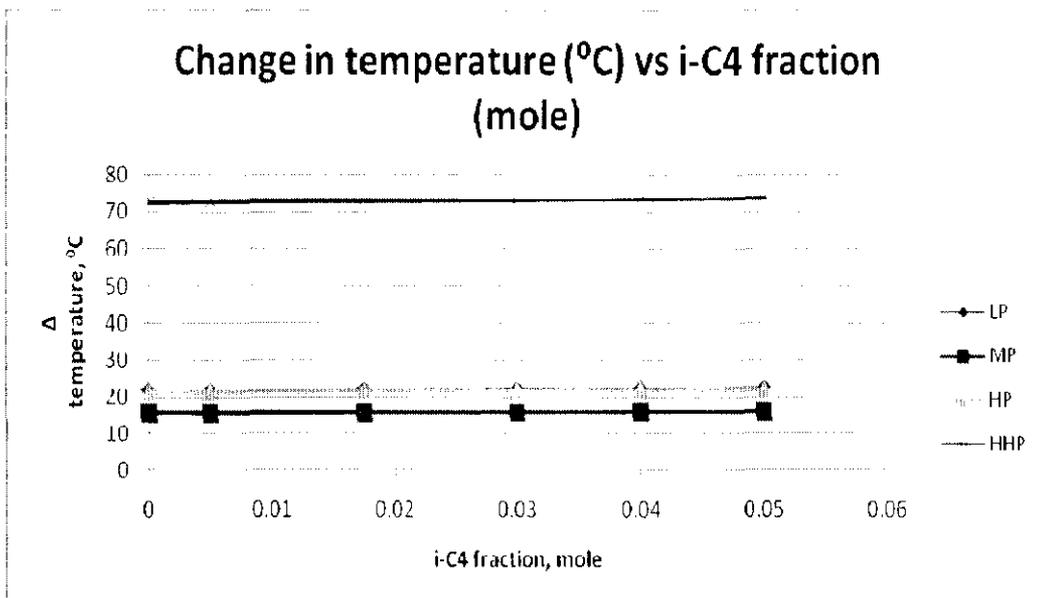
**Figure 35: Graph of change in temperature vs. i-C4 fraction**
