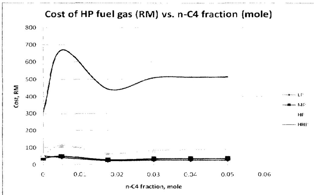
**Figure 45: Graph of cost of HP fuel gas vs. n-C4 fraction**
