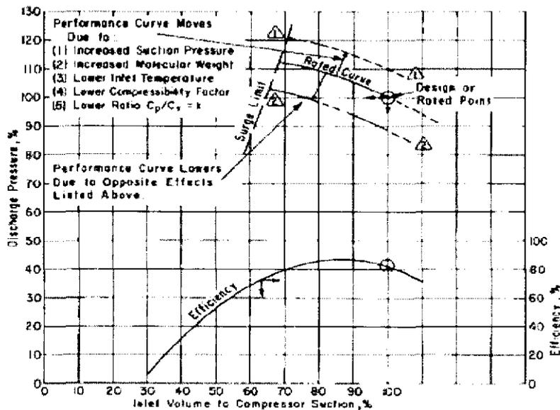
Figure 18: Compressor performance curve
