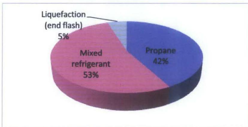
**Figure 17: Power consumption of different compressor in liquefaction process**
