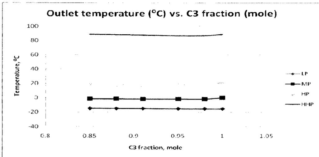
**Figure 26: Graph of outlet temperature vs. C3 fraction**
