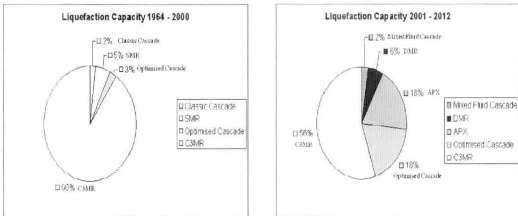
Figure 4: Evolution of LNG technologies; worldwide applied natural gas liquefaction technologies [4]
