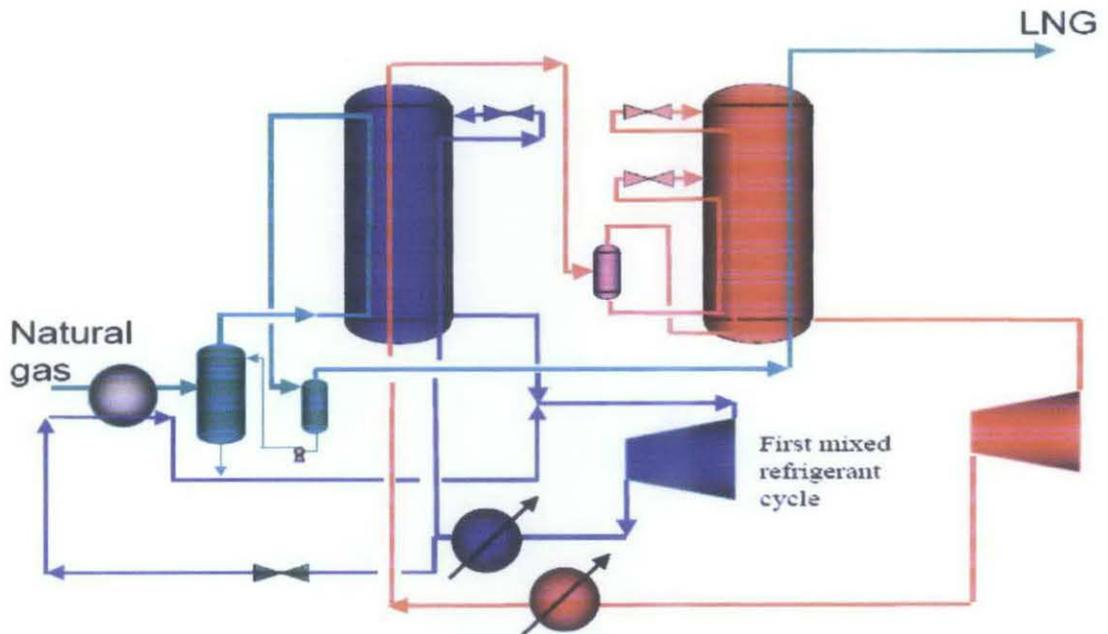
**Figure 9: DMR process flow**
