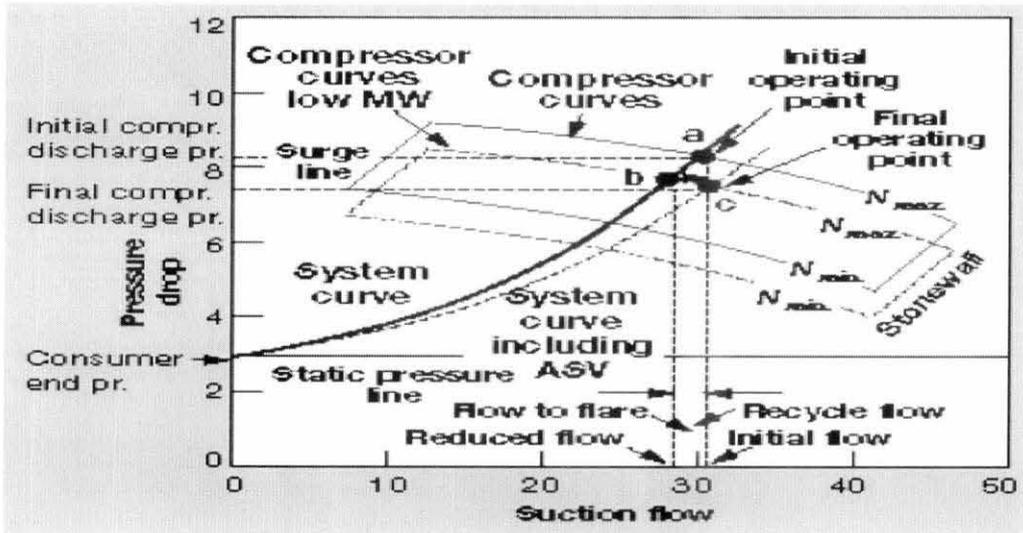
Figure 19: Molecular weight on compressor's operating curve
