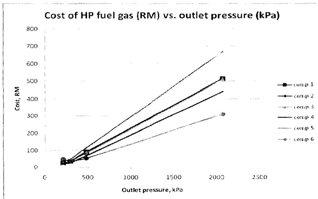
**Figure 47: Graph of cost of HP fuel gas vs. outlet pressure at different compositions**
