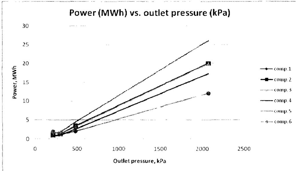
**Figure 41: Graph of power vs. outlet pressure at different composition**
