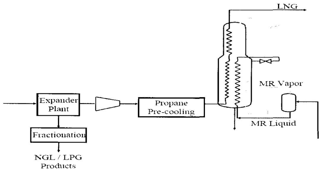
**Figure 10: NGL/LPG extraction before liquefaction unit**
