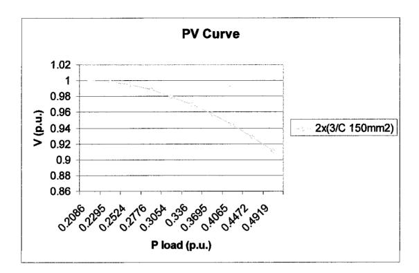
Figure 6 : PV Curve After Cable Size is Changed to 3/C 150mm<sup>2</sup>
