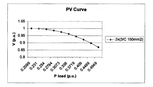
Figure 12 : PV Curve After Number of Transmission Line is Decreased
