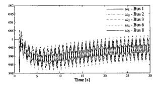
. Generator speed oscillations for the IEEE 14-bus test system due f bifurcation triggered by line ontage at 40% overload.
