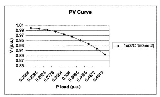
Figure 7 : PV Curve After Number of Transmission Line is Decreased
