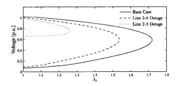
Fig. 10. Nose curves at bus 14 for different contingencies for the IEEE 14-bus test system.
