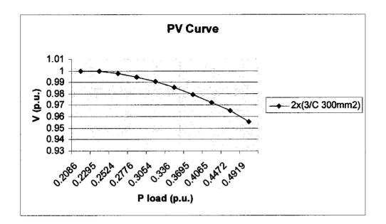
Figure 5 : PV Curve of Base Case Load Flow Analysis.
