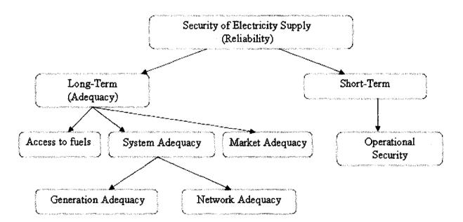
Figure 1 : Aspects of Security of Electricity Supply
