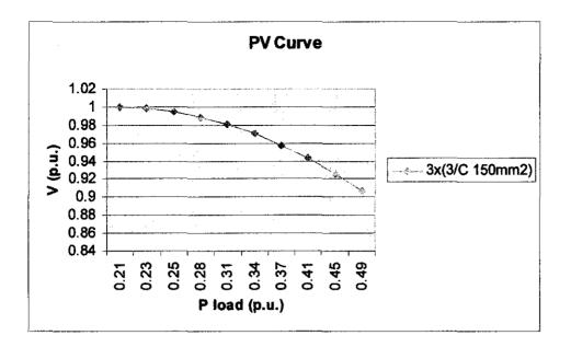
Figure 11 :PV Curve After Cable Size is Changed to 3/C 150mm<sup>2</sup>
