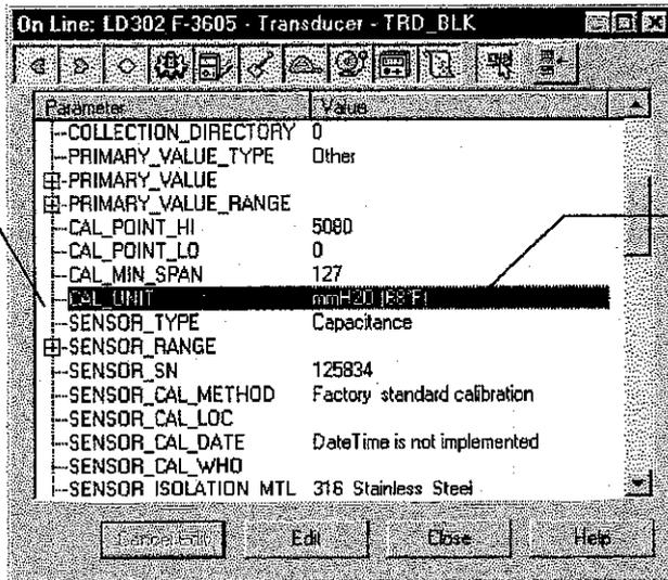
The appropriate calibration unit can be chosen by selecting the Engineering Units available for each type of Transducer Block.
