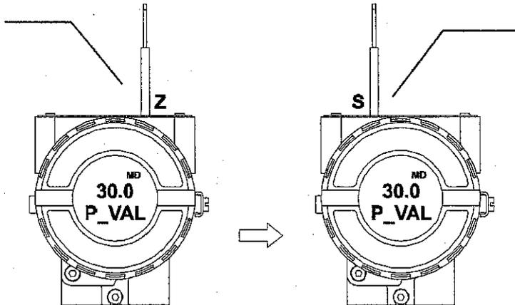
Place the magnetic tool in orifice S and wait during 5 seconds.
