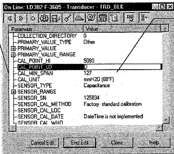
For its case, a sensor range 2 is used: The URL is 5080 mmH2O or 200 inH2O.
