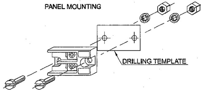
Fig. 1 - FIELDBUS FOUNDATION - BT302 - Mounting
