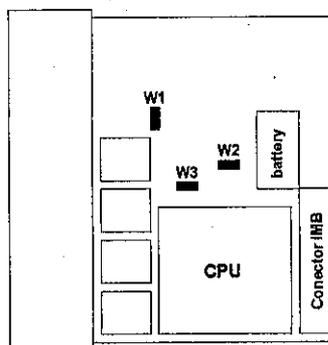
The W1 Simulate jumper must be ON to enable simulation in the Simulate (SIMULATE\_D or SIMULATE\_P) parameter of output and input function blocks.
