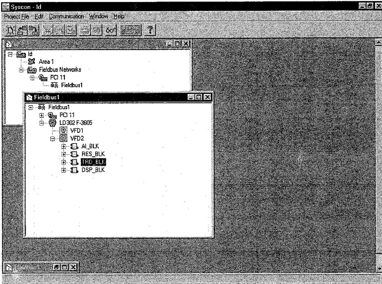
Figure 3.10 – Creating Transducers and Function Blocks
