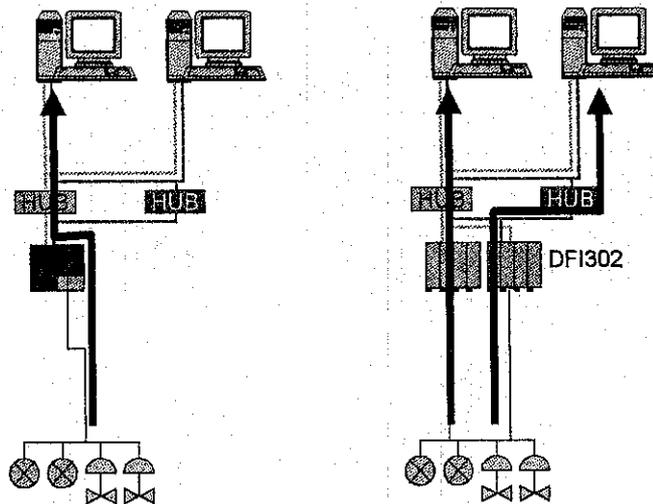
Typical versus Smar Solution: The DFI302 interface permits 2 redundant paths.
