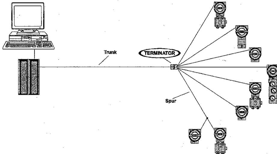
Fig. 2 - FIELDBUS FOUNDATION - Tree Topology
