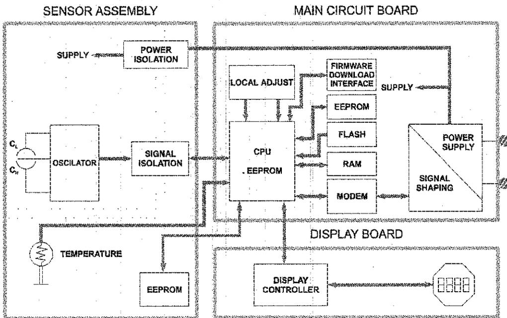
Figure 2.2 - LD302 Block Diagram Hardware
