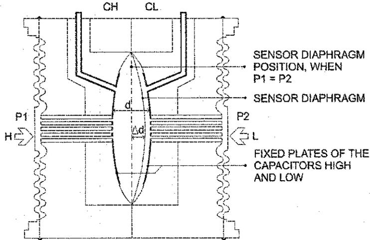
Figure 2.1 - Capacitive Cell
