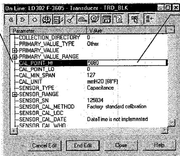
For its case, a sensor range 2 is used: The URL is 5080 mmH2O or 200 inH2O.
