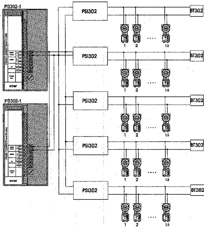
Fig. 1 – Connection Diagram of Fieldbus Elements to PS302-1
