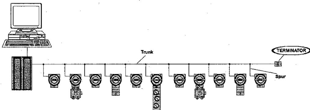
Fig. 3 - FIELDBUS FOUNDATION - Bus Topology
