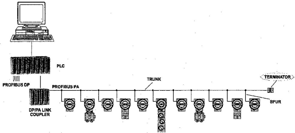
Fig. 4 – PROFIBUS PA – Bus Topology
