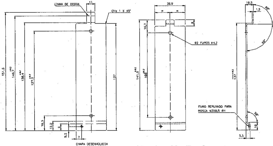
**Fig. 3 – Dimensional Drawing of Auxiliary Support**
