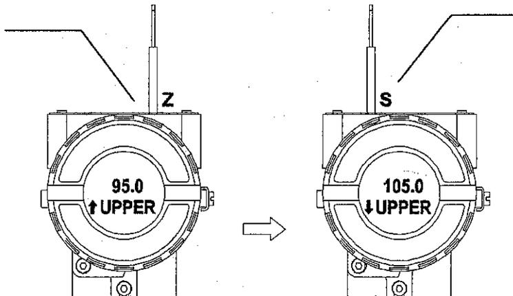
In order to decrement the upper value, place the magnetic tool in orifice Z to shift the arrow to the downward position and then, by inserting and keeping the tool in orifice S, it is possible to decrement the upper value.
