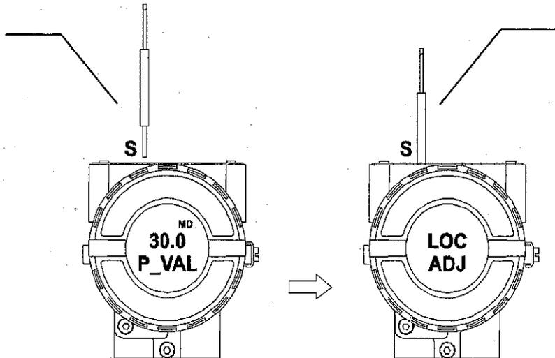
Insert the magnetic tool in orifice S once more and LOC ADJ should be displayed.
