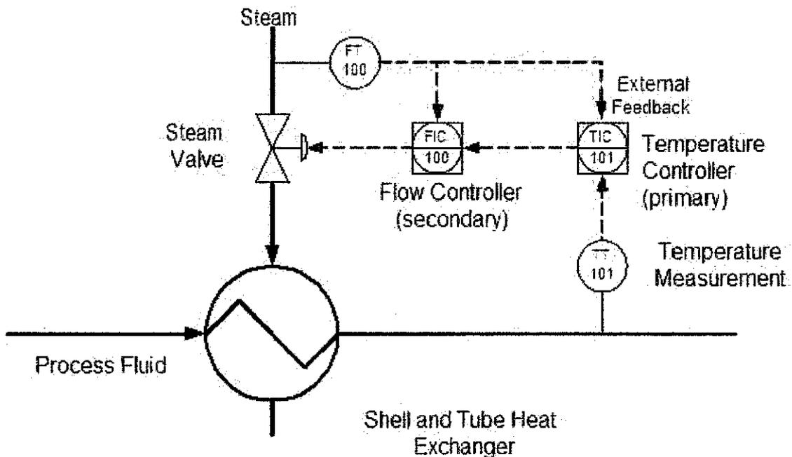
Figure 5 Overcome windup in cascade control
