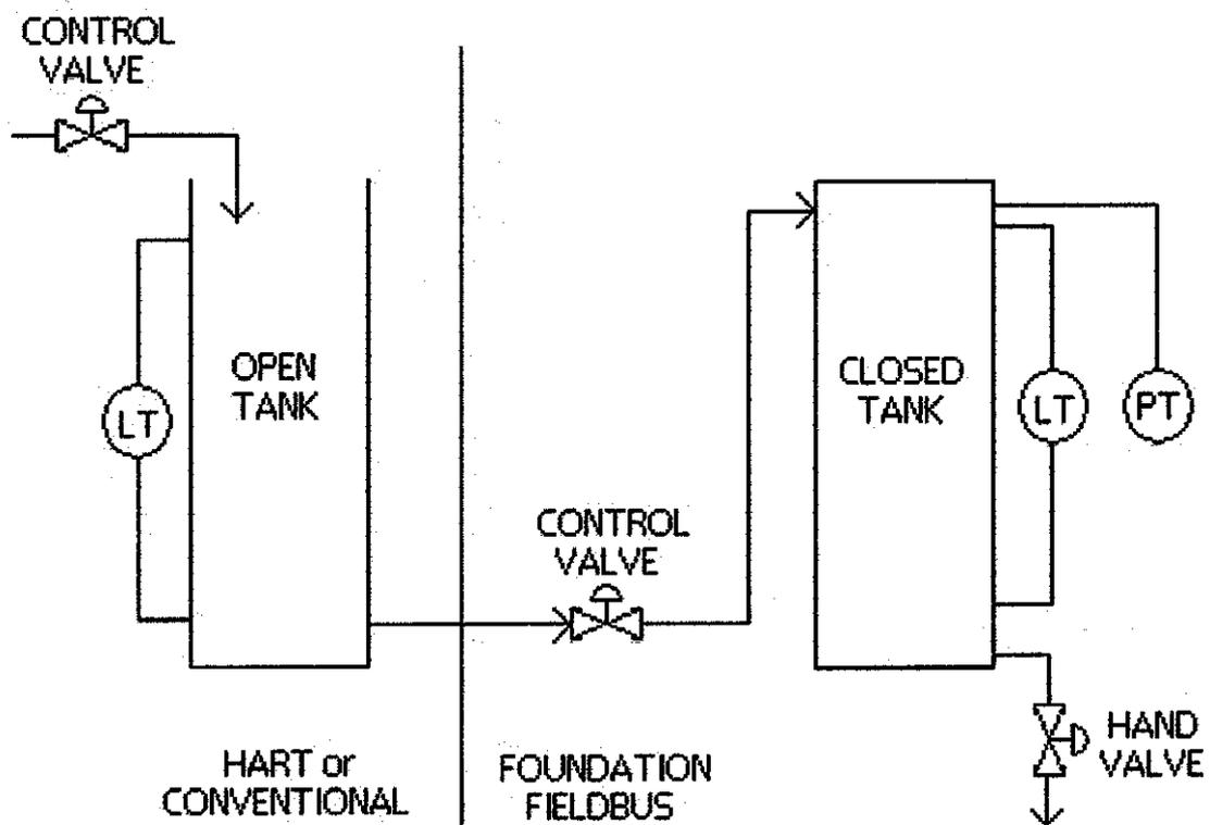
Figure 7 Fieldbus test platform design
