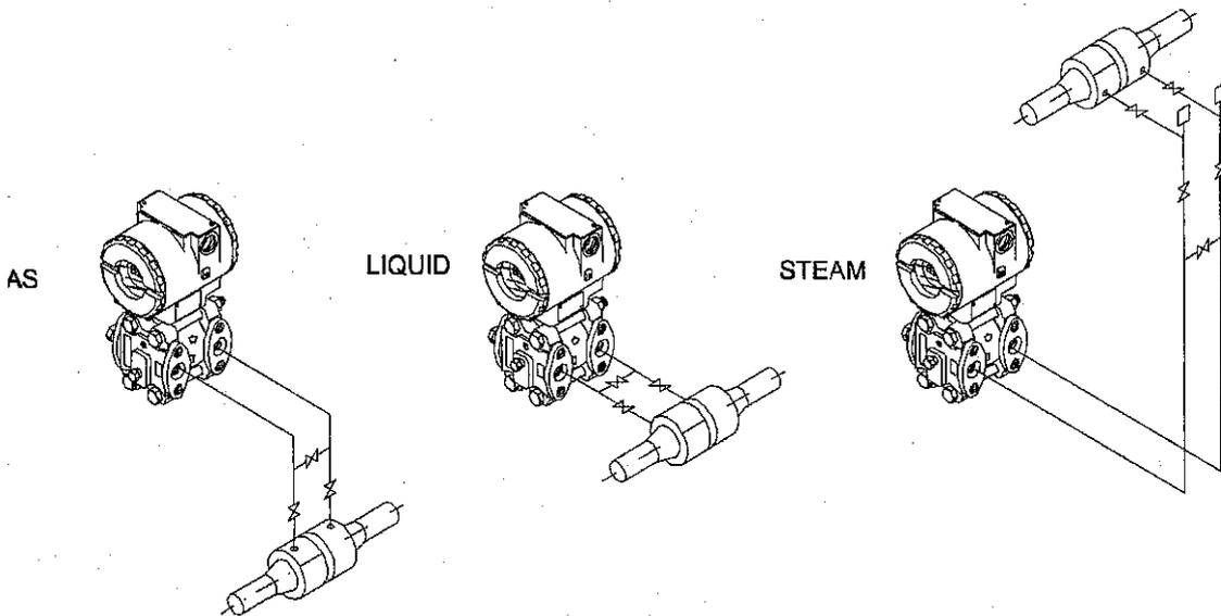
Figure 1.3 - Position of the Transmitter and Taps
