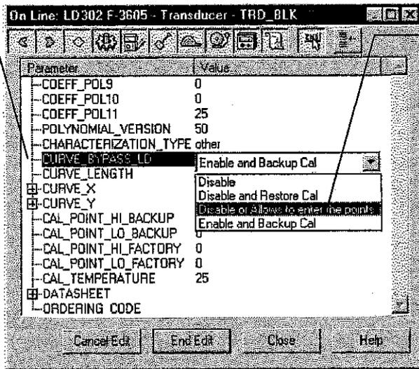
By the list box the user can enable or disable the Characterization Curve, enter the points, restore or backup the curve entered. This parameter should be used preferably by a method of calibration.
