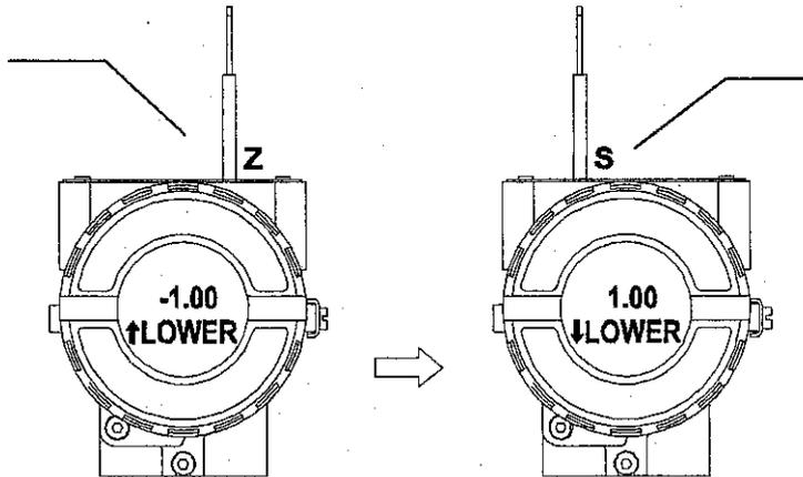
In order to decrement the lower value, place the magnetic tool in orifice Z to shift the arrow to the downward position and then, by inserting and keeping the tool in orifice S, it is possible to decrement the lower value.
