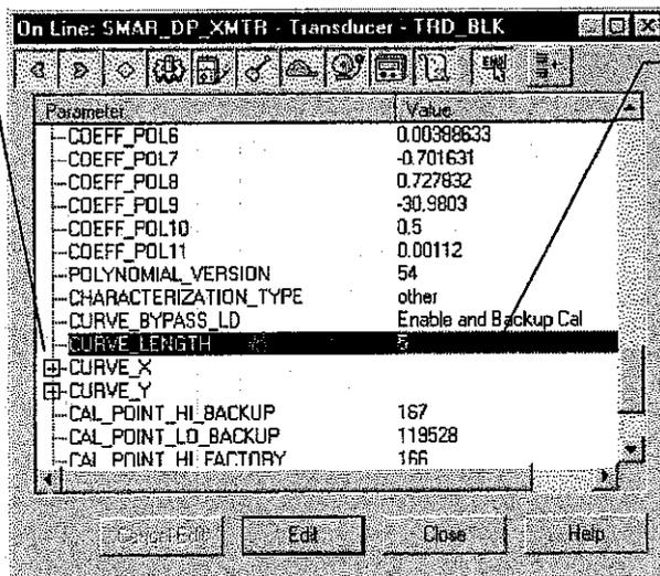
Its Characterization Curve can have a minimum of 2 and up to 5 points. These points should be between the calibrated range for better results.
