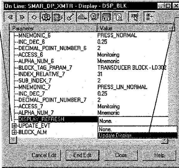
The option "update" should be selected in order to execute the upgrade of local adjustment programming tree. After its step all the parameters selected will be shown on the LCD display.
