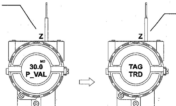
In this option the first variable (P\_VAL) is showed with its respective value (if you want that it keeps static, put the tool in S orifice and stay there).
