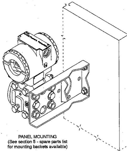
Figure 1.2 - Dimensional Drawing and Mounting Position for LD302
