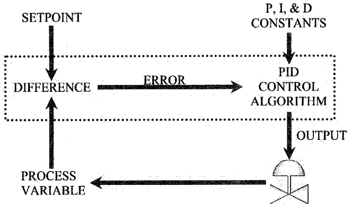
Figure 2 PID control
