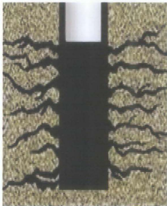
Figure 2: Acidizing cleans clogged channels
