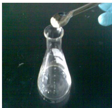
Mixing adsorbents into Pb(II) and Cd(II) Nitrate solution
