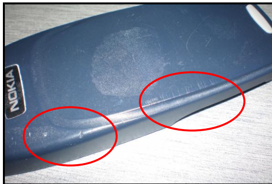
Figure 27: Scratches and Dents on Dummy test specimen casing
