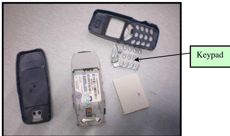
Figure 8: Different components of the drop specimen (Back view)
