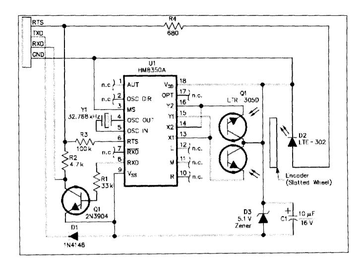
Figure 15: Schematic diagram of a conventional ball type mouse. The circuit consist of power input, input for X and Y axis motion signal, 3 button input (Left, Right and middle click), and three led source for generating the motion binary signal.
