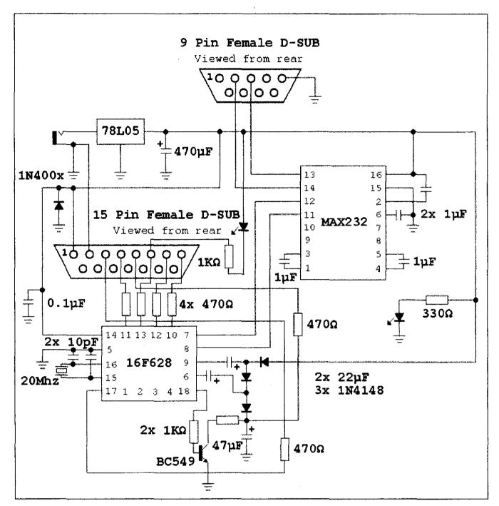
Figure 16: Microcontroller Programmer circuit schematic diagram. The circuit is use for programming the microprocessor controller for the pen shape mouse design circuit.
