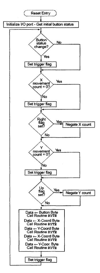
Figure 17: Flow Chart of Main Microcontroller program
