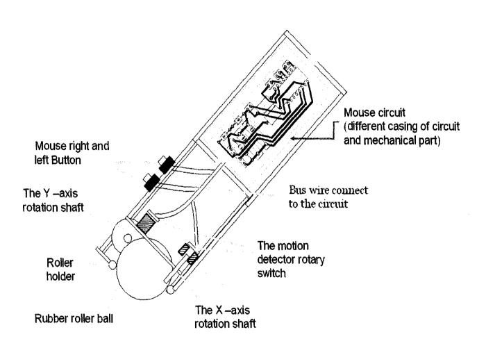
Figure 14: Improvement to Pen Mouse design 3 with roller holder. The project mouse model currently refers to this design. Due to its practical position of the shaft.
