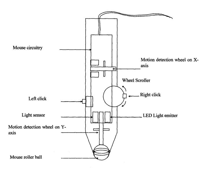
Figure 12: Pen mouse design 1 has unpractical shaft position that allows the ball to move in only one axis. The design is not selected to construct the pen shape mouse.
