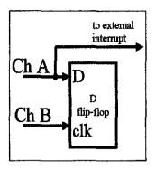
Figure 3: Flip flop for mouse encoder
