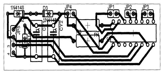
Figure 11: Schematic diagram of PCB circuit board
