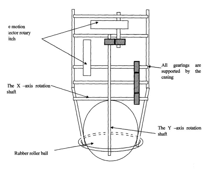
Figure 13: Pen Mouse design with mechanical gearing to move the encoder shaft for the photo sensitive to detect the waveform required for the computer to translate it in motion in x and y directions.
