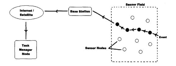
Figure 3.1: Basic Scenario for Area Monitoring
