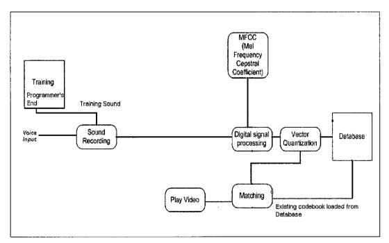
Figure 3.1.3-1: Data Flow Diagram
