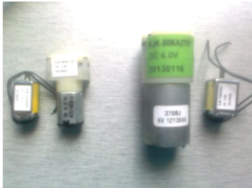
FIGURE 5 The motor pumps and air valve. The left side is the components rated at 3 VDC, and the right side is the components rated at 6 VDC.
