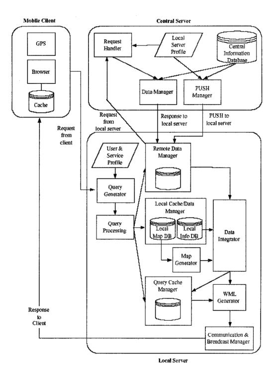
Figure 1 - System architecture for location based services.
