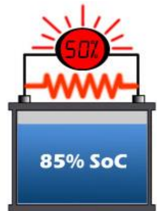
Figure 20: Inaccurate SoC reading by BCI standards
