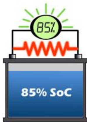
Figure 19: Accurate SoC reading by impedance spectroscopy
