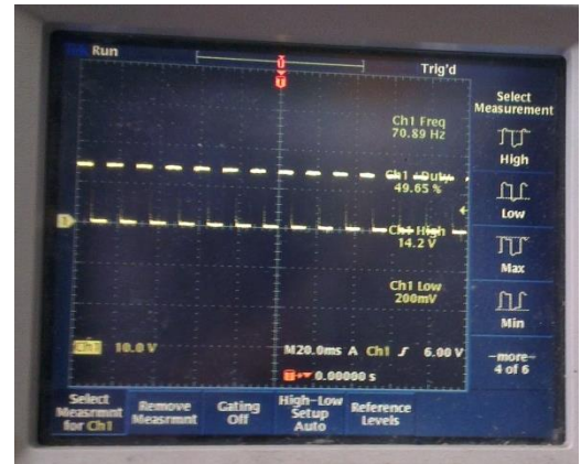
Figure 36: RPM output signal (70Hz at 2000rpm)
