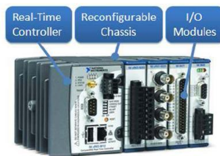
Figure 11: Main parts of CompactRIO
