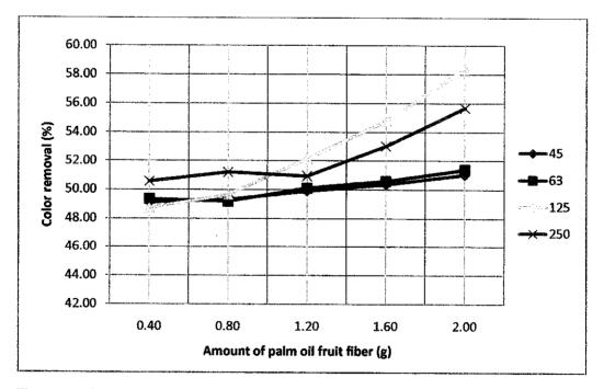
Figure 5.1 Color removal versus amount of palm oil fruit fiber for different particle size
