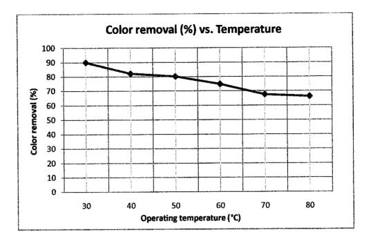
Figure 4.8 Color removals (%) versus different initial temperature
