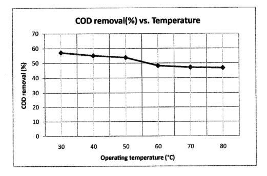
Figure 4.9 COD removals (%) versus different initial temperature
