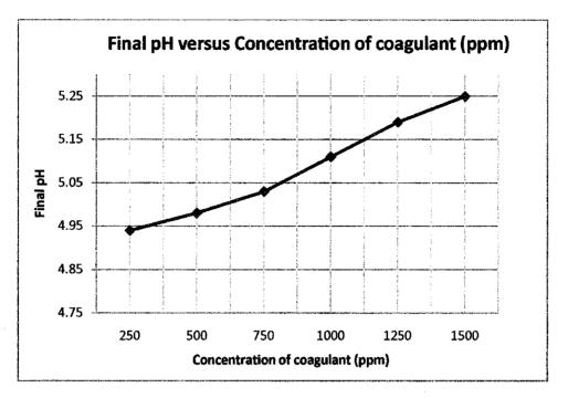
Figure 4.1 Final pH versus different concentration of coagulant
