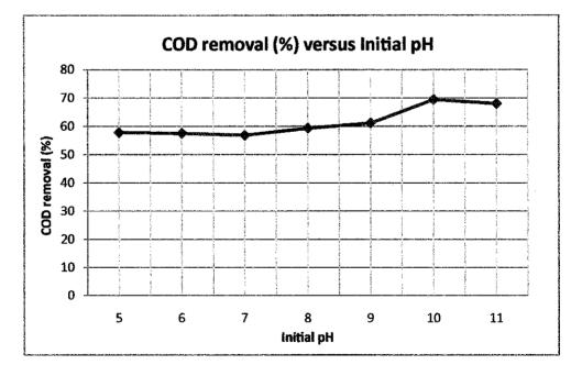
Figure 4.7 COD removal (%) versus different initial pH
