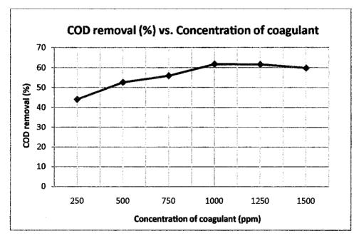
Figure 4.3 COD removal (%) versus different concentration of coagulant
