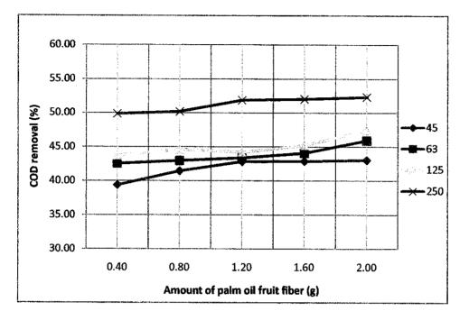
Figure 5.2 COD removal versus amount of palm oil fruit fiber for different particle size
