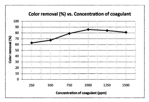
Figure 4.2 Color removals (%) versus different concentration of coagulant
