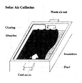
Figure 2.1: Single glazing solar air collector
