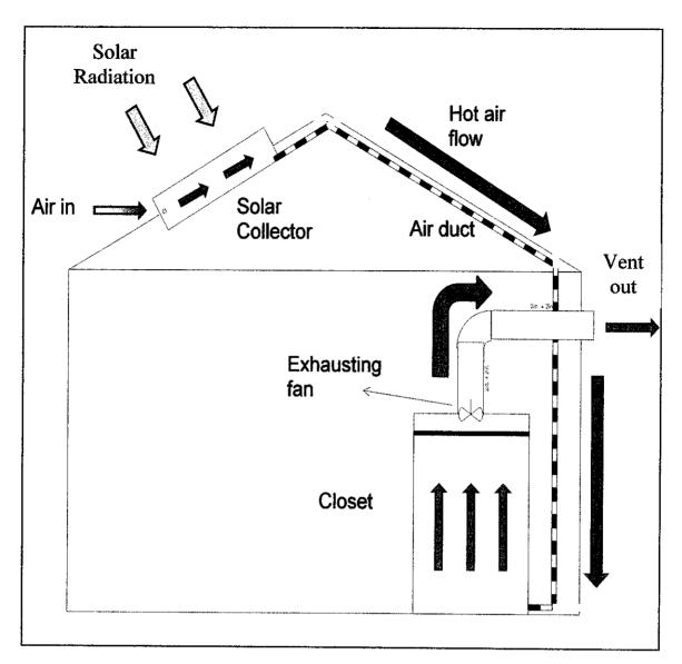
Figure 3.2: Schematic diagram of the Cloth Drying Closet
