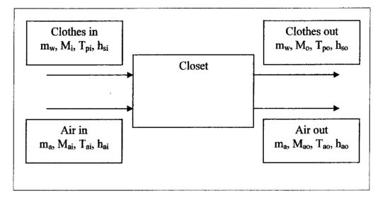
Figure 2.4: Schematic diagram of a drying process
