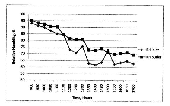
Figure 4.5: Graph showing variation of the drying closet inlet and outlet relative humidity with time of the day (November 11, 2008)
