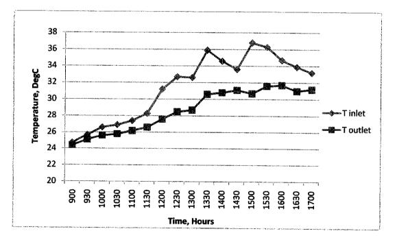
Figure 4.4: Graph showing the variation of the drying closet inlet and outlet temperature with time of the day (November 11, 2008)
