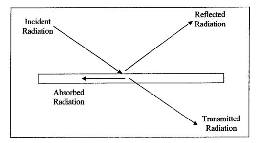
Figure 2.3: Distribution of Radiant Energy on a surface
