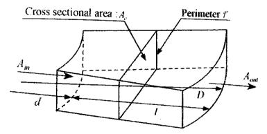
Figure 3.1: The geometry of a brake vane
