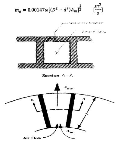
Figure 2.3: The airflow of the ventilated disc
