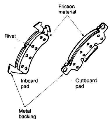
Figure 2.1: The parts of disc brake pads [8]
