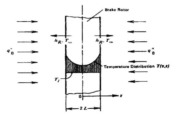
Figure 2.2: Thermal system representing brake rotor [10]
