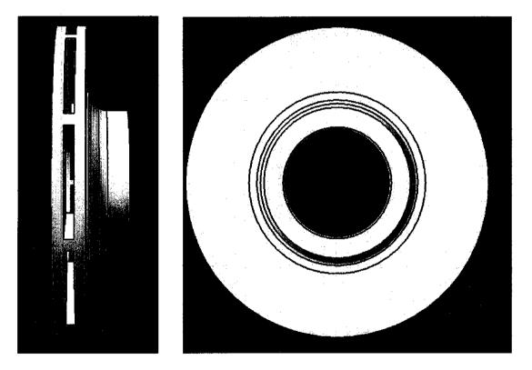
Disc brake system designs (disc) - front and right view
