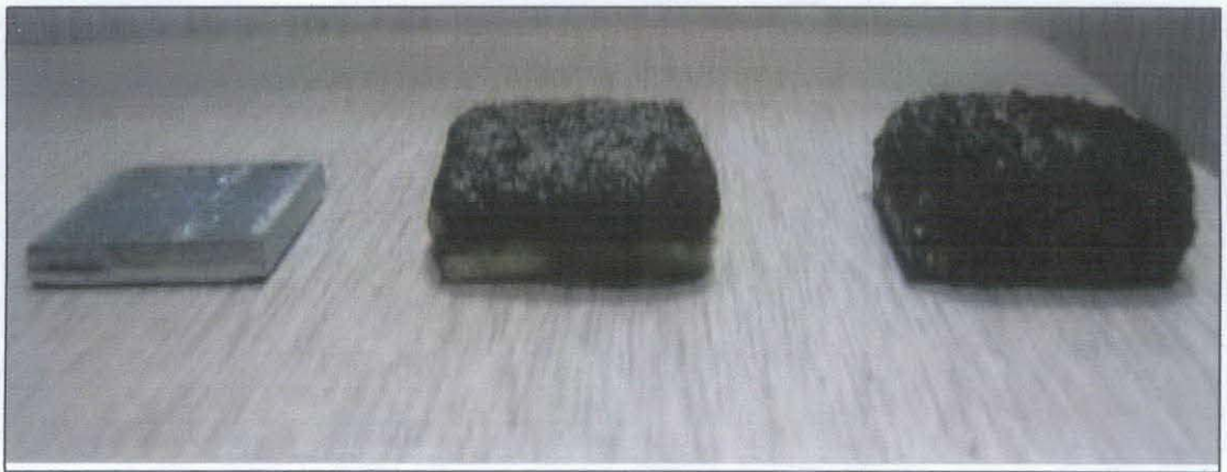
Figure 30: Side view of sample B after fire testing
