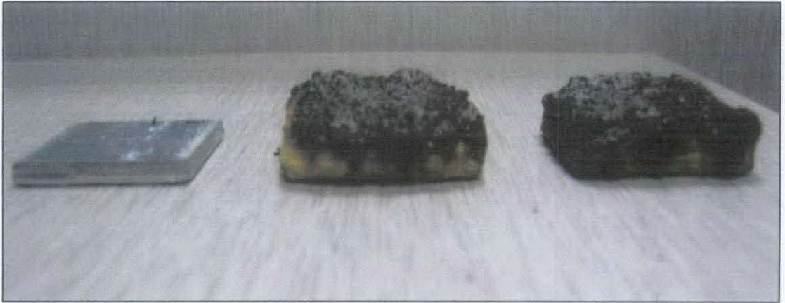
Figure 29: Side view of sample A after fire testing
