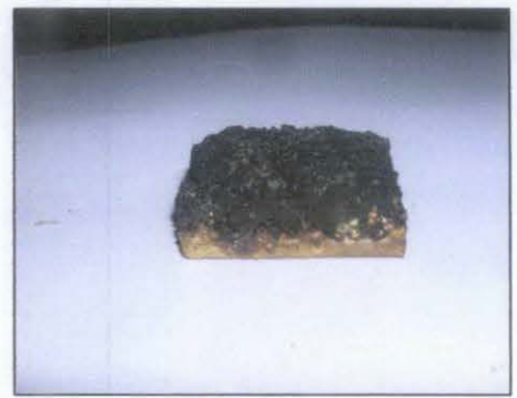
Figure 16: Sample B with fiber after exposing to fire for 10 minutes.
