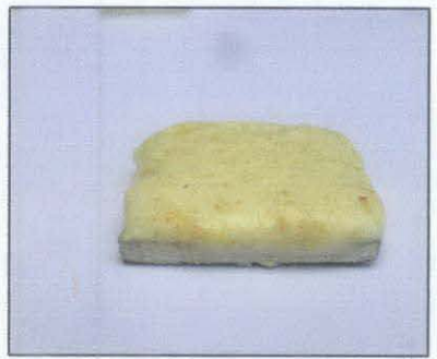
Figure 12: Sample B with fiber after cured.
