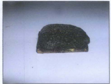
Figure 14: Sample A with fiber after exposing to fire for 10 minutes.
