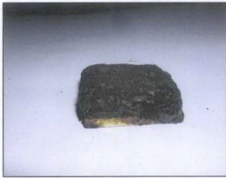
Figure 13: Sample A after exposing to fire for 10 minutes.
