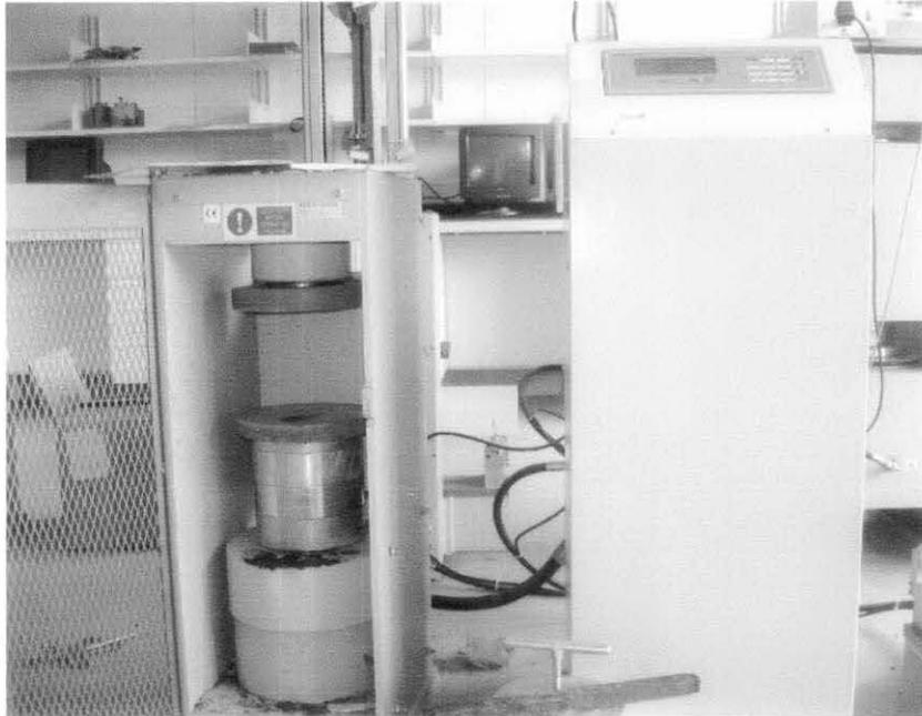
**Figure B1: Bench-Height Base Unit and Electrical Control System of Compression Testing Machine**
