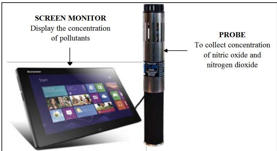
Figure 3.3: Toxic Gas Test Meter
