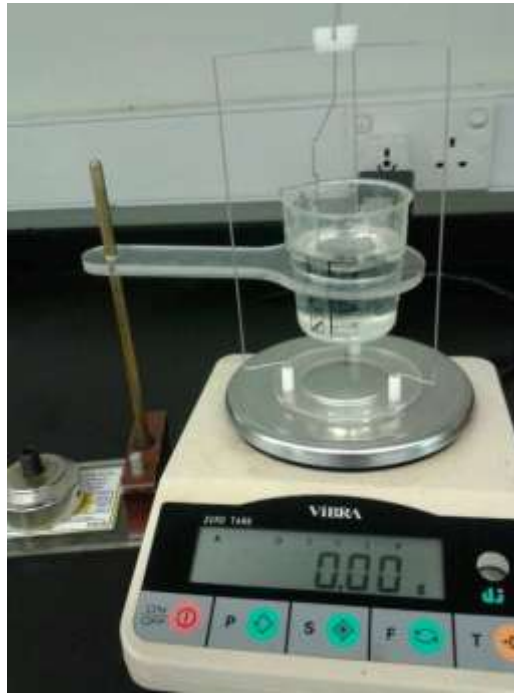
Figure: 3.9: Density test setup
