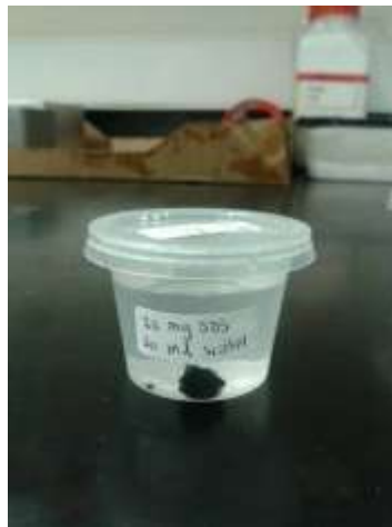
Figure 3.11: Dipping sample in the Sodium Lauryl Sulfate surfactant
